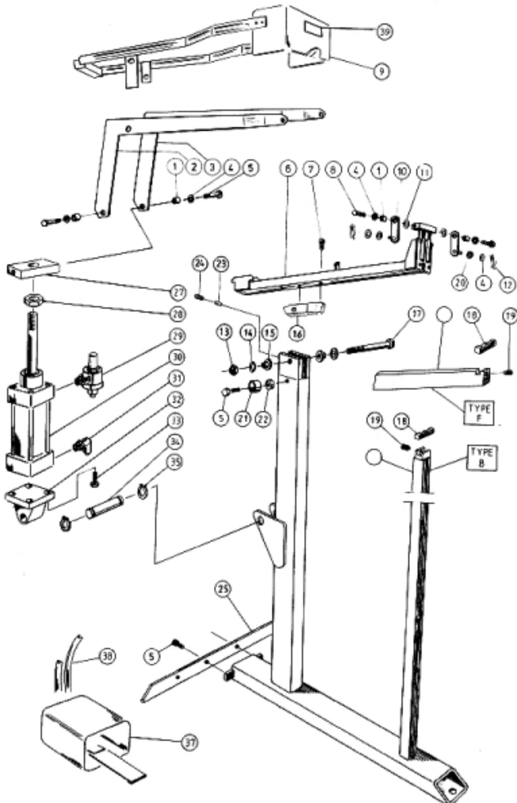
Spare Parts List Pneumatic Staplers type B and F with type 561 head
