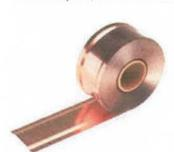
Roll staples are an excellent way to speed production when using packaging staples as a method of closure. The staples come in rolls of 1000 for hand tool use and 4000 for automated machinery. This provides fewer changes for the operator. They are equally secure to a "C" staple. Packaging staples provide the most secure closure of cartons available. The Bostitch roll type staple is used specifically in Bostitch tools.
