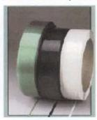
Polyester strapping is for bundling much heavier loads than polypropylene. It is much stiffer and less flexible. Some polyester banding can be used in place of steel strapping. Polyester has the advantage of not rusting or staining. Polyester strapping is available in machine and hand grade.
