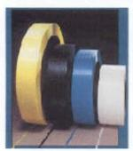
Hand grade polypropylene strapping is commonly used to secure palletized material or for bundling of packages. The strap may be tensioned by hand or other types of tensioners. It can be sealed with either a metal buckle or seal. Common specifications to check are footage per roll, core size and break strength.
