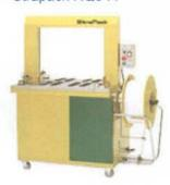
The RQ8-A series is designed for high output operations. The strap automatically feeds through the arch. There are many different arch sizes to fit a wide array of products. The RQ8-A differs from the RQ8 in that it has a conveyor top for the automatic movement of product through the arch. The RQ8-A has the ability to automatically triggered for operator free use. This machine is available for regional delivery.
